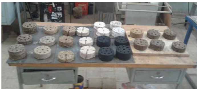
(a) Produced Priquette from Carbonized and Uncarbonized biomass.
